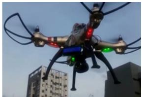
Another Civil Engineering student, Mr. Sadun Kodikara, using a drone, an Arduino Uno board, a digital camera, batteries and a Sonar sensor had invented a 'Digital Flying Staff' which can measure relative distances or heights that are beyond the bounds of human reach by sending a wave towards the desired object. This mechanism allows the device to calculate the distance or
